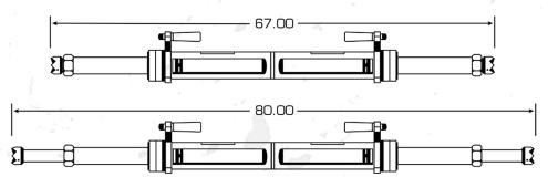
Designed to be used with either the P-25 or P-40. In combinations these extenders can supply you with up to a 10 ft. extension.
